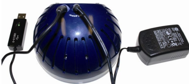
Fig. 1: Rear side of the Wöhler CDL 210 with USB cable and power supply
