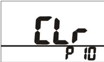
Fig. 17: Setup - Delete all records, Display 1
