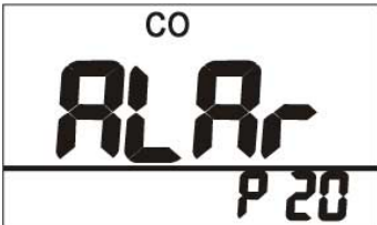
Fig. 19: Setup - Setting the CO Alarm Threshold
