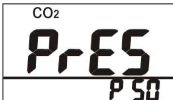
Abb. 23: Setup – Luftdruck, Display 1
