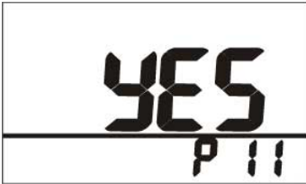
Fig. 18: Setup - Delete all records, Display 2
