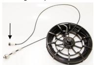
Fig. 57: Viper removed from the case. monitor plug covered by a lid
