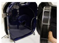
Fig. 56: Removing the viper with the connection cable from the case.
