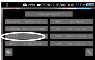
Fig. 49: Settings menu - wlan0\_IP is marked
