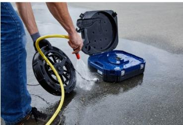
Fig. 58: Cleaning the viper and the rod
