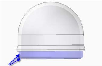
Fig. 51: Fitting the camera dome
