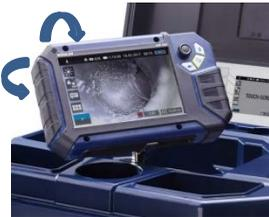
Fig. 10: You can turn and tilt the monitor
