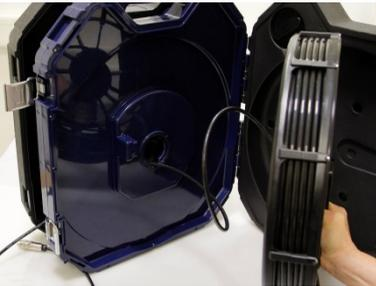
*Fig. 56: Removing the viper with the connection cable from the case.*
