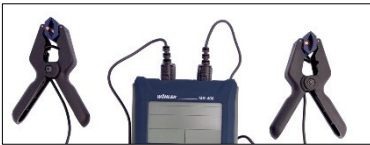
Fig. 19: Connection of the temperature clamps
